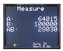
The Tausand Abacus AB2502 device, has 2 input channels. Its measure menu shows the last measured value of single counts of each channel, A, B, and the coincidences detected for the pair AB.
