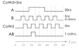
Coincidence window 5ns. A single 20ns pulse arrives on port A while a burst of 5ns pulses at 100MHz arrives on B. Only 1 coincidence is detected, corresponding to the pulse in A arriving within the same coincidence window with the second pulse in B.
