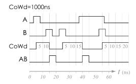
Coincidence window 1000ns. In this example, although a long coincidence window of 1000ns is set, during a lapse of 75ns two valid coincidences arrive and are correctly detected.
