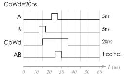
Coincidence window 20ns. Two 5ns pulses arrive in A and B within the coincidence window. Therefore 1 coincidence between A and B is detected.
