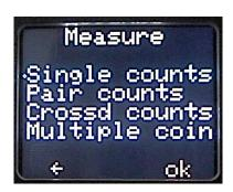
Since every experiment is different, and even within the same experiment there are different stages where some information is more relevant than another, the Tausand Abacus AB2504 offers different ways to read the measurements live of its 4 input channels. They are categorized in: single counts, pair counts, crossed counts and multiple coincidence counts.
