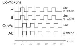
Coincidence window 5ns. Synchronized bursts of 5ns pulses at 100MHz arrive at both input ports, A and B. Every couple of pulses is considered a coincidence, and therefore a total of 100MHz coincidence rate is achieved. This is the limit case of maximum repetition rate for the Tausand Abacus AB1004.
