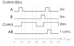
Coincidence window 20ns. Two 5ns pulses arrive in A, and one 5ns pulse arrives in B. The pulse on B arrives too late to be considered a coincidence with the first pulse from A, but is close enough to the second pulse in A, arriving about 5ns later, to be considered a coincidence with it.
