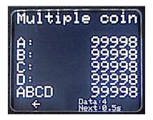
Shows the last measured value of single counts in every channel, A, B, C and D, and the multiple coincidence counts as configured in the settings menu.
