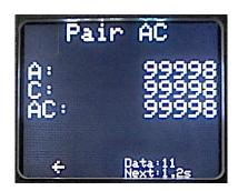
Shows the last measured value of single counts in a selected pair of channels, and their corresponding 2-fold coincidences.
