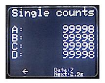
Shows the last measured value of single counts of all 4 channels: A, B, C and D.
