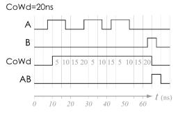
When several pulses arrive at the same port, let us say A, before the coincidence window timer is done, each new pulse resets the coincidence timer allowing an auto-extend of this timer expecting for a detection on the other port, let us say B.
