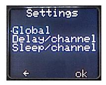
Select the category with the rotary selector, and enter the submenu with the 'ok' (right) button.
