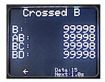
Shows the last measured value of single counts and 2-fold coincidences containing a selected channel. For example, if the selected channel is C, the measurements shown in the screen are C, AC, BC and CD.
